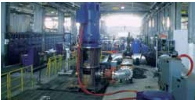
We recently achieved the important objective of fitting every Unit with a modern Testing Room: in our plants in Gessate and S. Mauro Torinese we can test pumps with powers up to 650 kW, capacities up to 8000 m<sup>3</sup>/h and pressure values up to 120 bar. Our plant in Taglio di Po has been designed for sealless pumps intended for applications in the chemical sector.
